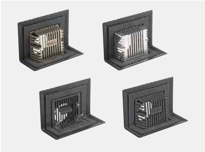
The Harmer cast iron Two-Way outlet is unobtrusive and suitable for use in a parapet wall construction. It can be used vertically or horizontally for connecting to 50, 75 and 100mm pipework making it suitable for use in balcony installations. A choice of flat or rectangular grates design is available in cast iron, nickel bronze or aluminium.
