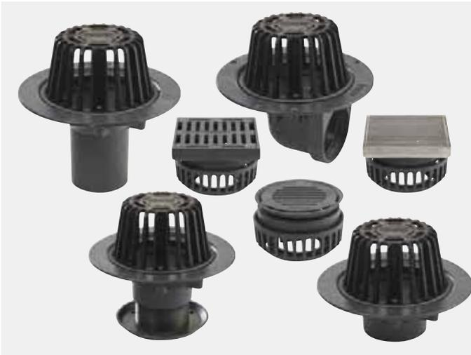
The Harmer cast iron medium sump range is a compact outlet body in vertical and horizontal variations for connection to 50, 75 and 100mm pipe work. Vertical bodies come with either spigot or threaded outlets and horizontal body versions are available in threaded only. A comprehensive range of grates is available for use in different types of application including load bearing circular and square grates which are suitable for areas with vehicular access.
